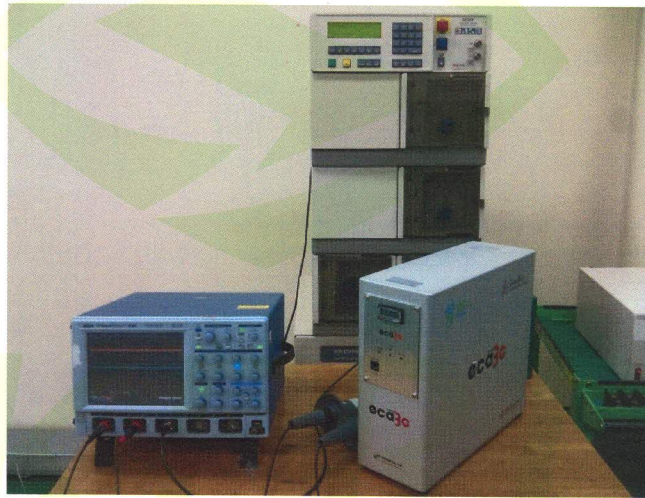
Photo. SG03 : Measurement of the front of wave sparkover voltage test
